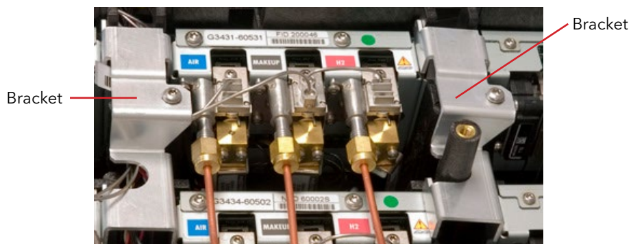
Figure 3.21. Locating the EPC Module Brackets
